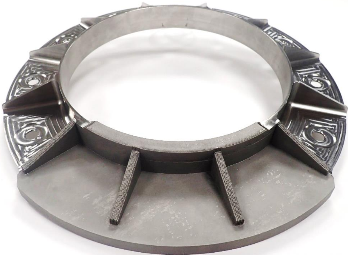
Aerospace flange in Ti6Al4V Built using DED, heat treated and partially machined
